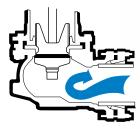
CLOSED The main valve held closed by operating nut & water pressure; barrel is dry.
