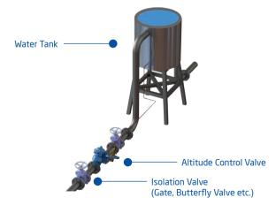
Armaş Altitude Control Valves control the water volume without float in an elevated tank.
